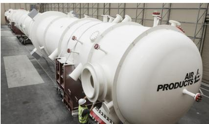
Liquefaction processes and equipment: Air Products offers a full range of liquefaction process options (see back page). Whether you require only a few tons per hour or millions of tons per year. Air Products has the process and equipment to serve your needs. In addition, and depending on the process, Air Products' equipment and supply may include our MCR® coil wound heat exchangers, cold boxes, and cryogenic turbomachinery including hydraulic turbines.
