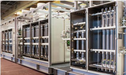
Air Products' Membrane Solutions provides technology and equipment for on-site nitrogen generation in a wide range of energy industry applications including floating LNG platforms. These membranes have proven their durability during years of use in refineries, petrochemical plants and gas fields. Our nitrogen membranes satisfy the industry's need with a reliable high purity nitrogen supply that is mobile, low maintenance, scalable and flexibly configured.
