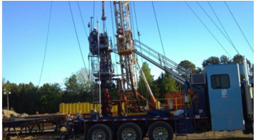
**Nitrogen improves the safety of snubbing operations by providing an inert blanket to prevent development of hydrates in blowout preventers and surface lines.**
